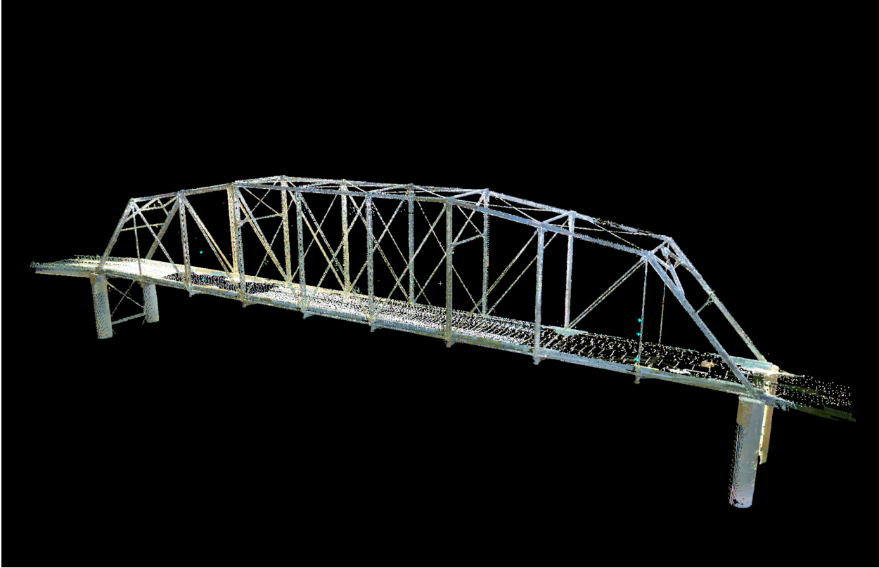
Figure 5. Point cloud from Ward's Crossing Bridge scans.
