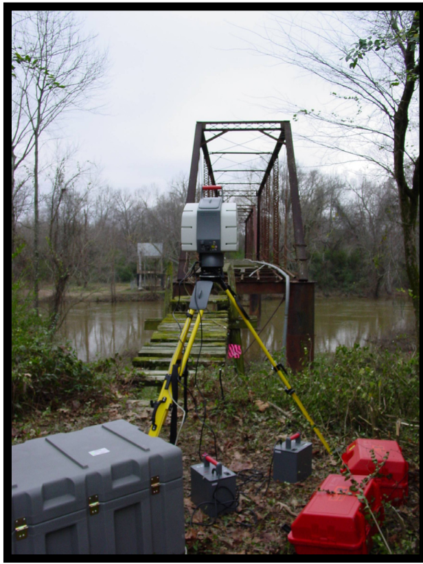
Figure 4. Scanning the Old River Bridge
